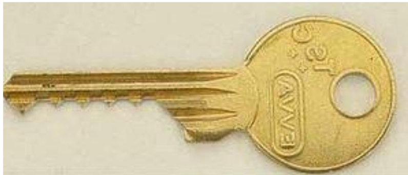
Above: a typical bump key
